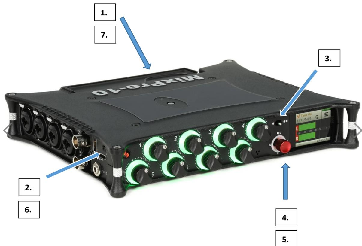
1. Insert a SD card on the back side
